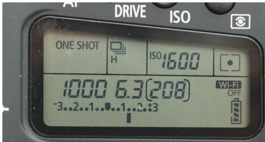
Figure 8. The meter reading on the top of my Canon 80D (same as the scale shown in the bottom of my viewfinder). The current reading shows the exposure is about one and a third EV over-exposed. (One EV is the equivalent of a doubling or halving of light reaching the sensor).
