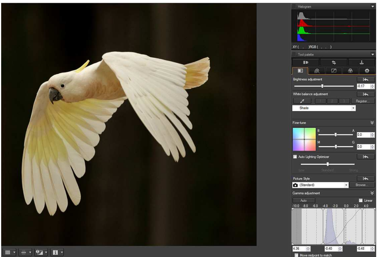
Fig. 5(b). The white balance has been set to 'shade' making the image appear too 'warm'. The correct white balance is 'cloudy' corresponding to the conditions on the day the image was captured.
