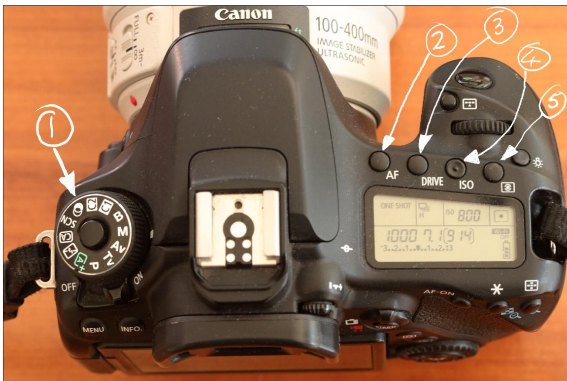
Figure 1. Controls on the top of my Canon 80D: (1) is the mode dial, currently set on Manual; (2) is the Auto Focus (AF) mode setting, currently on One Shot as shown on the LCD panel below this button; (3) is the Drive mode which determines whether the camera takes a single shot or multiple shots each time the shutter button is pressed, currently set on high speed continuous; (4) is the ISO setting button, currently set on ISO 800 (when this button is pressed, the ISO can be changed by rotating the dial visible just above it); (5) is the metering mode, currently set on centre spot metering as shown on the LCD panel just below the button.
