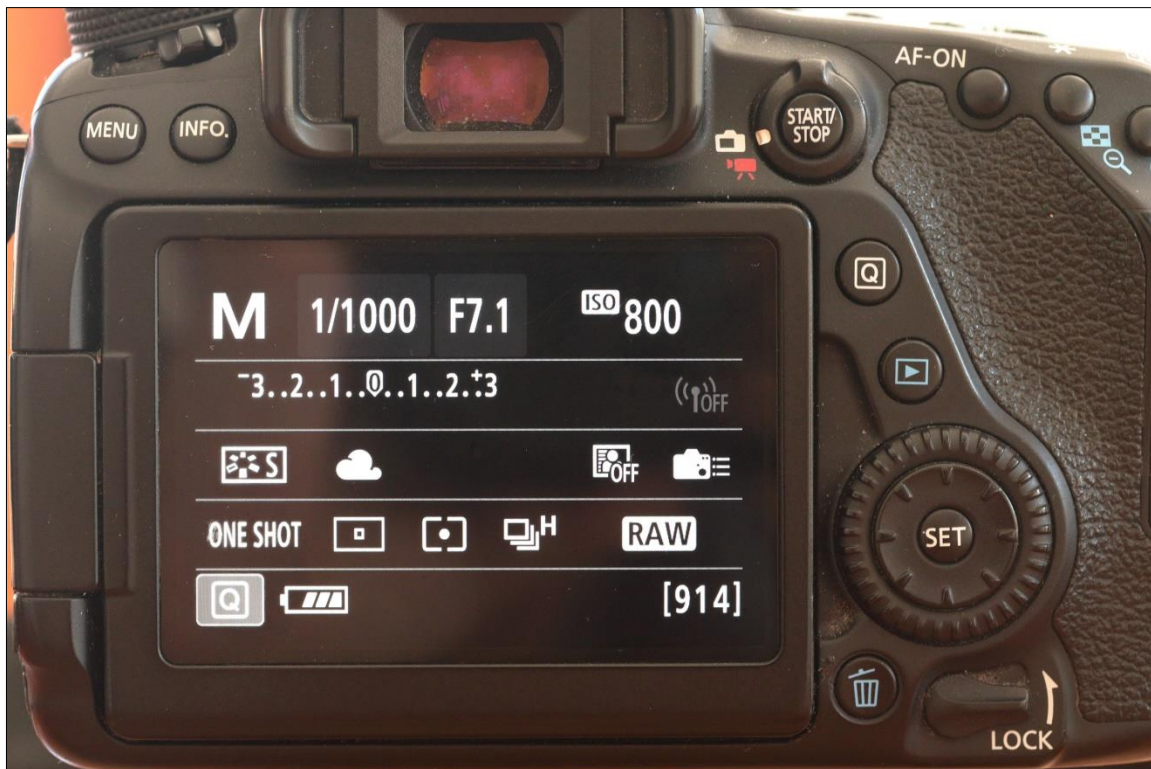
Figure 2. The display panel on the back of the camera, also showing current settings. On some cameras, this is the main screen that is used for these settings as some cameras don't have an LCD display panel on the top of the camera (as shown in Figure 1). This is also the screen where menu items are displayed after pressing the 'Menu' button (top left). There are a few additional items on this compared to the LCD panel on the top of the camera. On the first line, the 'M' shows that the mode dial is set to 'M' (manual exposure). The second line shows the exposure compensation (beyond the scope of this article). The third line, from left to right, shows the Picture style (S=standard), the current white balance setting (cloudy), the automatic exposure adjustment setting (off – beyond the scope of this article) and the control to customise the camera's buttons (camera specific and beyond the scope of this article). The fourth line shows the AF mode (One shot), the focus point selection (single point), the exposure point selected (centre point), the Drive mode (multiple shots taken when shutter button pressed) and the file recording mode (RAW). The last line simply provides information on the battery and remaining shots.
